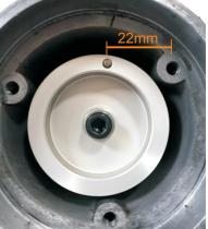
Important! Check that the face of the rotor is 2mm(+/-0.6) below the deck that the stator sits on.
