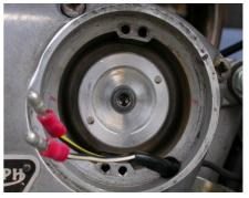
Install the Tri-Spark rotor using the correct socket head bolt for your engine. Two bolts are provided for use with the earlier and later engine models. When tightening the bolt ensure that the bolt is sufficiently tight to pull the rotor completely onto the taper inside the cam. When fully tightened the step surface on the back of the rotor should be touching the face of the cam.
