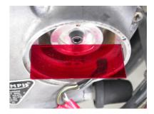
Install the stator unit using the original pillar bolts and washers. Additional washers are provided in case the pillar bolts bottom out before they tighten on to the stator. Do not tighten the pillar bolts as this time.
