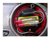
When reinstalling the points cover a small piece of foam should be positioned over the wires to stop them vibrating as shown in the above photograph
