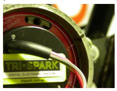
Now mark the engine casing adjacent the CW mark on the outer rim of the stator unit, then remove stator unit.
