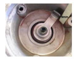
Fit the Tri-spark rotor as shown in the above photo and tighten with the socket head bolt and washer supplied. Be certain that the rotor is located correctly, there should be a 9 to 11mm gap between the edge of the rotor and the casting as shown above.
