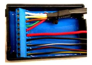
Notice that the fuse is in the negative power lead to the box (positive ground installation). This is unconventional in electronics but this way it protects to output transistors best against faults in the coils and wiring. If the fuse blows, check that the coils are not shorted in the primary and that there are no short circuits to the frame in the coil connections from the trigger box.
