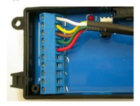
Connect wiring from the trigger box to ignition coils and wiring harness. Fit cover on Tri-Spark trigger box and fix in position. Connect the wiring as shown in the following photo and wiring diagram (see below).
