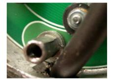
Use the washers provided to space out the pillar bolts. Watch for contact here. Apply some silicone between the wire and the pillar bolt at the end of the installation to stop any chaffing.
