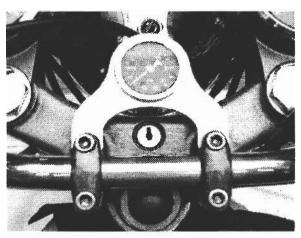
Loosen the four socket head cap screws that secure the handlebars. Next, slide the oil pressure mounting bracket between the upper and lower handlebar clamps as shown in the picture at the left. Tighten the front two socket head cap screws first. Make sure the oil pressure gauge bracket is clamped securely before tightening the rear socket head cap screws. Tighten the two rear socket head cap screws. This part of the assembly is complete.
