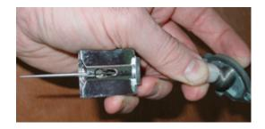
Now insert the end of the cable so that the nipple sits in its place in the throttle slide, Fig.5
