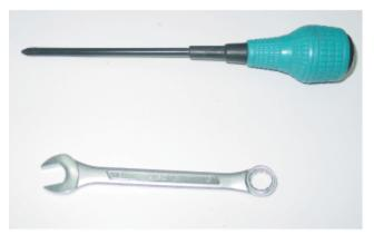
Screwdriver - used for removing the top housing of the throttle slide to attached the throttle cable.
