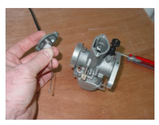
Having removed the top cover, push the nipple end of the throttle cable through the top cover and down the center of the spring and through the white retaining collar. Compress the spring and hold it all together so as much of the cable is showing as possible, Fig.4
