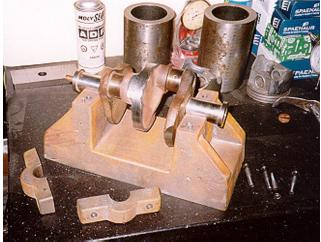
Figure 2 – Crank and fixture
