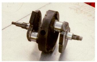
Figure 3 – The first crankshaft – original flywheel mounting holes are not used..
