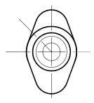
MODIFIED TRIUMPH INTAKE/ EXHAUST CAM AS VIEWED FROM TIMING SIDE
