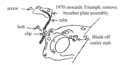
Ignore breather instructions for BSA and pre-1970 Triumph twin. 1970 on Triumph needs to have new breather hose fitted by drilling and tapping timing plug at back of crankcase and fitting hose. (With PCV valve for best breathing.)
