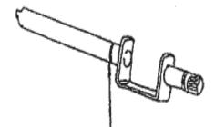
For left hand shift TR7/T140, machine o-ring groove, if not there, to retain oil in gearbox.
